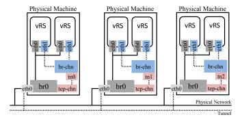
Fig. 7. Network Setup for VNF Chaining
